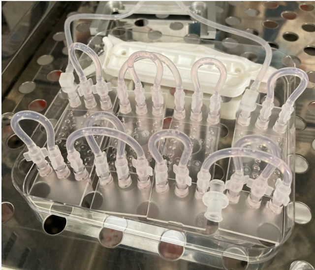
Four serially connected \mu -Slide Spheroid Perfusion, connected to the ibidi Pump System.
